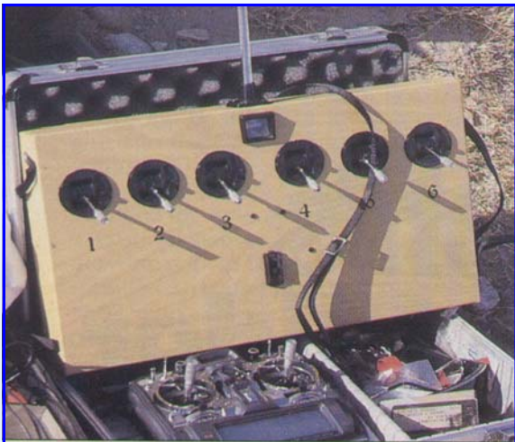
The Dornier uses a separate radio system to control the six engines; each engine can be controlled independently by the flight engineer by means of this special transmitter devised by John Wisniewski. John was the pilot for the flight, Bill Reed was the flight engineer.
