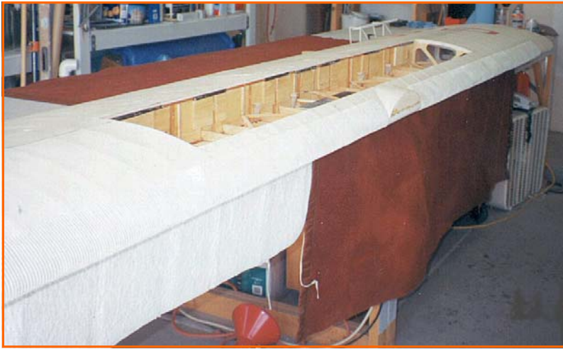
Wing showing opening for engine module as its being built in the photos at the right.
