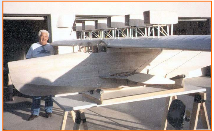
Looks like Marshall Sims is checking for a straight leading edge. Wing being fitted to check out fuselage seating..
