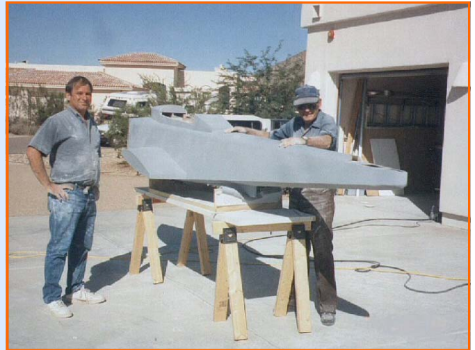
After 2 coats of fiberglass, each heavily sanded. Later sprayed thinned latex paint for the primer.
