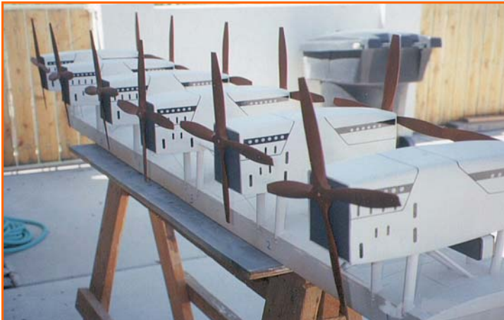
The engine module shown with static props and 6 1.6 hp Zenoahs
