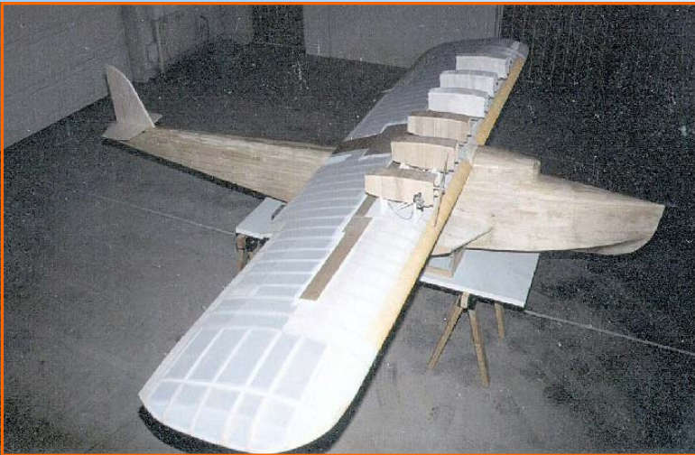
Here we see some of the engines nacelles partially finish and the wing covering.
