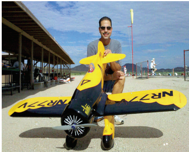
Wingspan: 70.9 in (180 cm) Overall Length: 46.6 in (118.3 cm) Flying Weight: 10.6–11.5 lb (4.8–5.2 kg) Engine Size: 1.20 cu in 2-stroke, 1.50 cu in 4-stroke Radio: Minimum 4 channels Servos: 6 servos (JRPS821 recommended) Wing Loading: 28.1–30.7 oz/sq ft Mike Marranca
