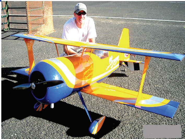
My Qui Que 85" wingspan Pitts Python. . BME 116 engine Mejzlik 28 x 10 prop. Spektrum AR9100 receiver and JR 8711 ser- vos all around. Eric Sauley
