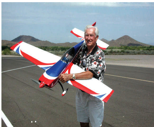
Wingspan: 70.9 in (180 cm) Overall Length: 46.6 in (118.3 cm) Flying Weight: 10.6–11.5 lb (4.8–5.2 kg) Engine Size: 1.20 cu in 2-stroke, 1.50 cu in 4-stroke Radio: Minimum 4 channels Servos: 6 servos (JRPS821 recommended) Wing Loading: 28.1–30.7 oz/sq ft Mike Marranca
