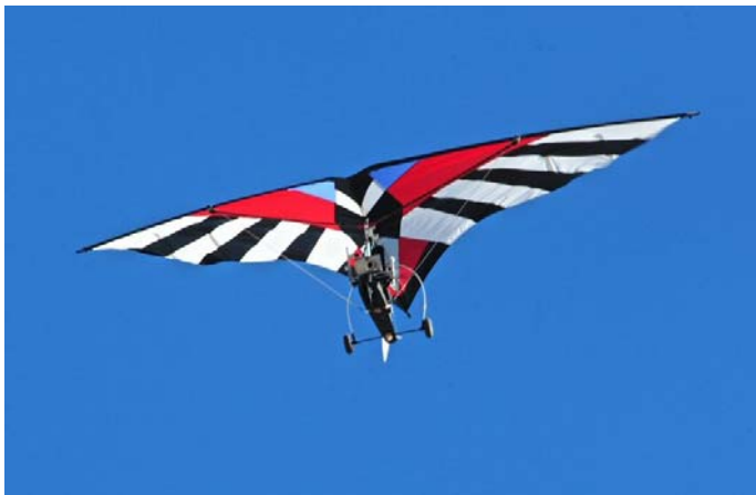
DAG REEVES HAWKEYE W.S. 92" W.A. 2200 sq.ft. 0-10 MPH Brushless motor 30/40A ESC 3-6 Chans. 15-20 mins flight time Cannon Powershot PHOTOS TAKEN BY THE HAWKEYE SEEN HERE
