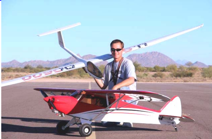
DUSTIN YOUNG MULTIPLEX DG 600 3.3 meter retract fiber glass fuse - Obeachie wings covered with white Ultra coat-uses spoilers and flaps for landing-.J/R 9303 with sailplane program using full span cambering.
