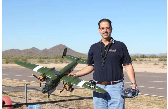
MIKE MARRANCA Hobby Lobby B-25 Apache Retractable landing gear and wheels (pre-installed) 2 brushless outrunner motors - 3 landing gear door sequencers 2 30A ESC- 3-Cell 2200 mAh 11.1V Lipo -10 servos - Navigation lights SEE MORE PHOTOS in this issue.
