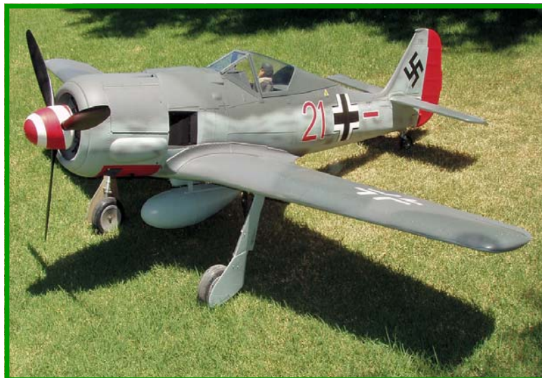
Tony Quist Airworld ARF, 102" Wingspan, Moki 250cc Radial, Futaba FASST Radio with Smartfly Competition 12 PowerSystem. Go to the VIDEO page and see Tony fly the FW190. Thanks Tony
